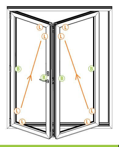
Liniar load bearing platforms **must be used** to keep door square and level.
